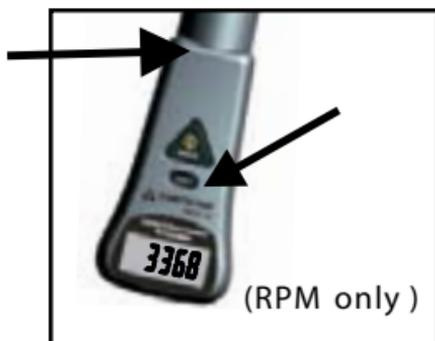
**Step 5:** Hold the meter and point it toward the rotating object targeting the reflective tape. Keep the targeting distance within 5 to 30 cm (2 to 13 inch).
